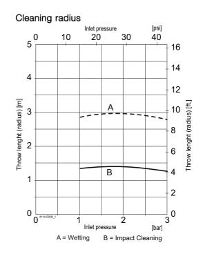
For Clip-on models, the flow rate is increased by approx. 0.5 m<sup>3</sup>/h. **Note:** The inlet pressure has been taken immediately before the inlet to the machine. In order to achieve the performance indicated on the curves, the pressure drop in the supply lines between pump and machine must be taken in consideration and the water temperature during testing was approx. 20°C.
