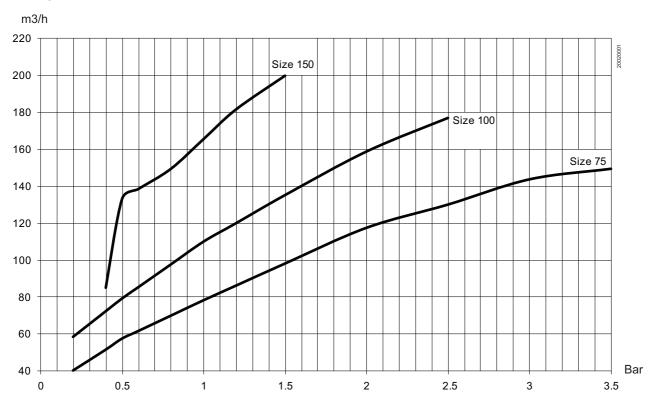
In accordance with EN 4126-1 Capacity measured at:  $\Delta P=10\%$  Set pressure  $\geq$  1 bar  $\Delta P=0,1$  Set pressure < 1 bar Medium: water (20°C)
